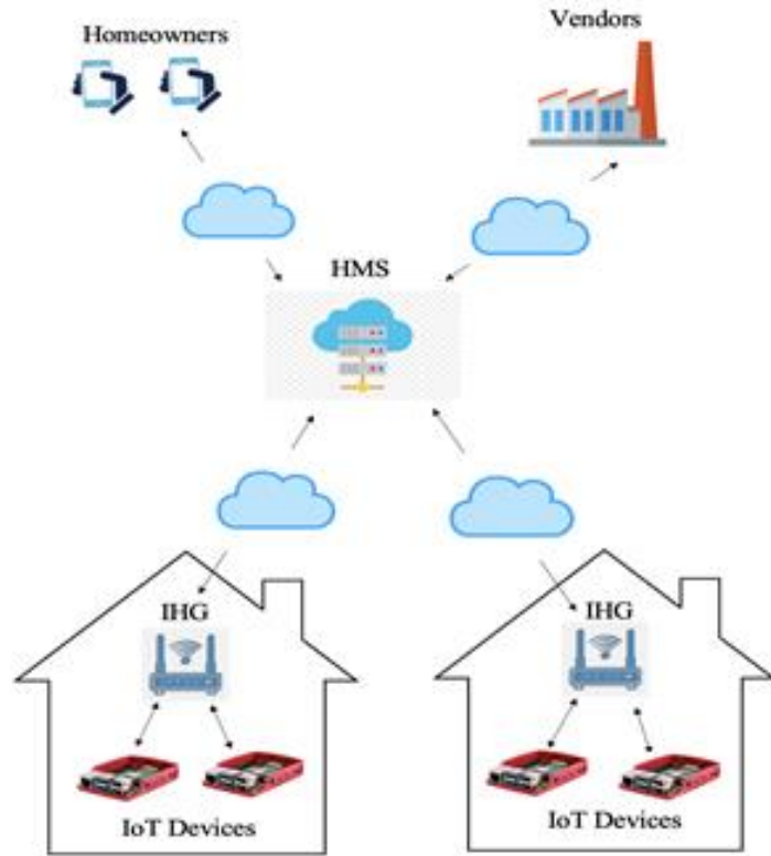
Overview of the Home Automation System architecture
